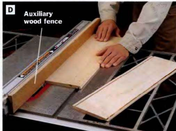
PHOTO D: Cut the bottom rabbet into the lower edge of the box sides. Attach an auxiliary wood fence if you use a table saw and dado-blade set to cut these rabbets.
