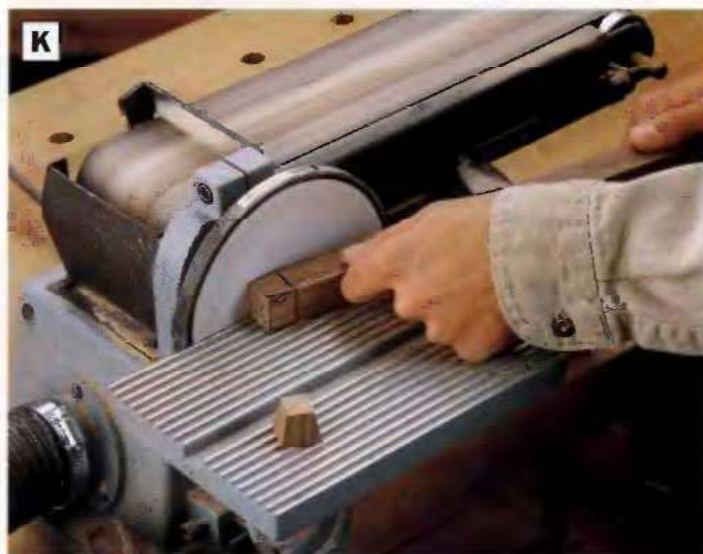
PHOTO K: For safety and to maintain control over the workpiece, sand the tapers on a long walnut blank, then cut off a foot and repeat for the other three feet.
