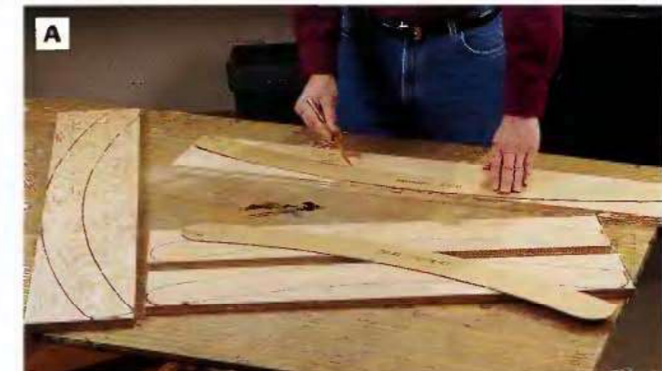
PHOTO A: Create seat and back support templates from hardboard, and use these templates to draw the profiles on the back and seat support workpieces (use treated lumber, not plywood as shown). Cut out the parts with a jig saw.
