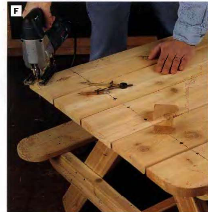
PHOTO F: Mark a 2¾-in. radius on each of the four corners of the tabletop, and trim the corners with a jig saw.
