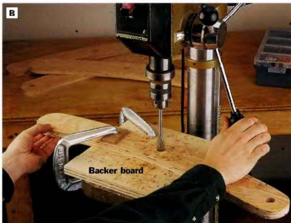
PHOTO B: Bore the \frac{3}{4} -in.-dia. leg pivot and lock dowel holes in the legs. These holes must be drilled straight through the legs, or the dowels will be difficult to align during assembly. Bore the holes with a drill press, or mount your drill/driver in a right-angle drill guide. Set a backer board beneath each workpiece before you drill, to keep the bit from tearing out the wood as it exits.
