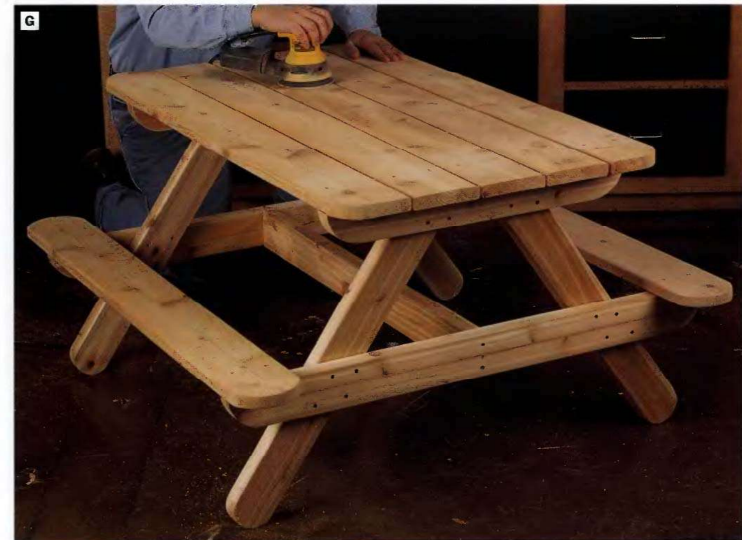
PHOTO G: Since cedar is prone to splintering, you'll want to give the table a good sanding to break the edges and smooth the parts. A random-orbit sander is the best tool for the job. It's a good idea to wear a dust mask when sanding cedar; the dust can be a respiratory irritant.
