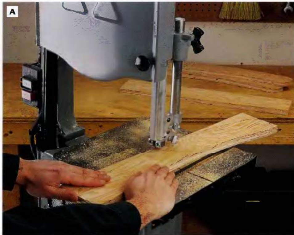
PHOTO A: Lay out and cut the four table legs on the band saw or with a jig saw. Since the profiles of the legs match, mark and cut one to serve as a template for tracing the profiles onto the other three leg blanks.
