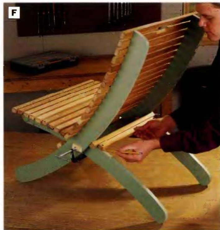
PHOTO F: Slide the seat assembly into the back assembly and use C-clamps to hold the chair together. Set the short crossbar against the lower long crossbar, mark its position, and install it with screws.
