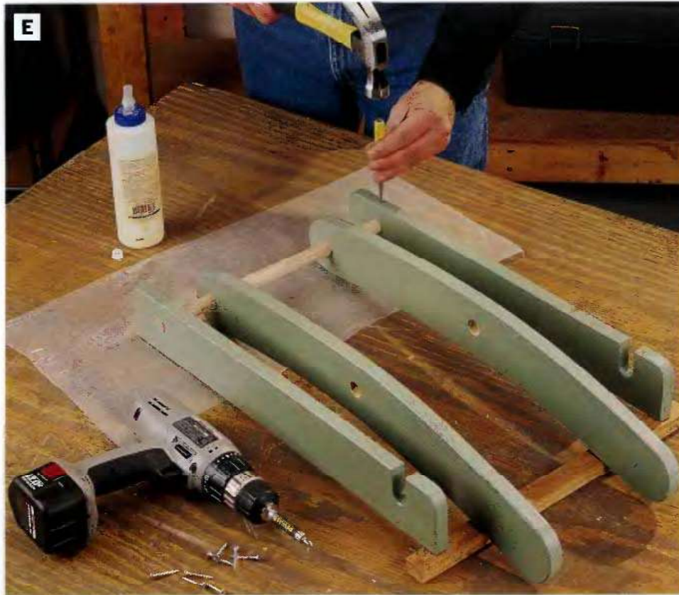
PHOTO E: Attach the first tabletop slat to the stretchers with screws. Lay the outer legs between the stretchers, and slide the table pivot dowel through the stretchers and outer legs. Pin the dowel in place with glue and finish nails driven into the dowel through the stretchers. Do not glue or nail the outer legs to the table pivot dowel.
