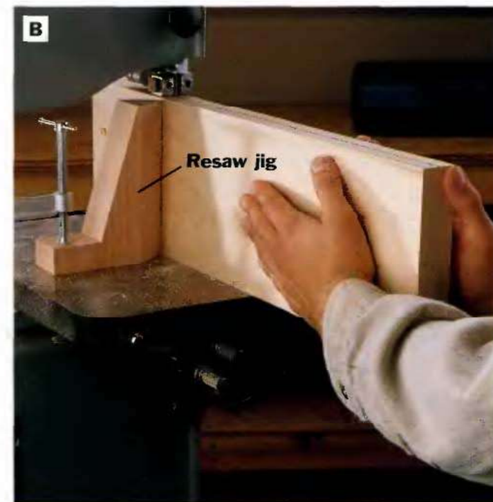
PHOTO B: Resaw the maple stock in half for the sides and ends of the box, using a marked centerline as a guide for the blade. A shop-made resaw jig clamped to the saw table will help square the board to the table and keep the blade tracking along the cutting line.
