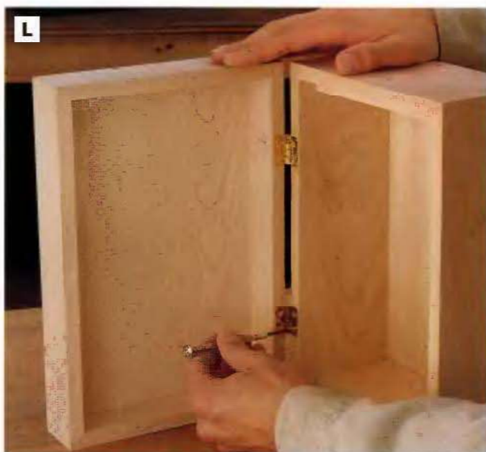
PHOTO L: Measure and cut the hinge mortises with a wood chisel, then install the brass jewelry box hinges to attach the lid to the box.
