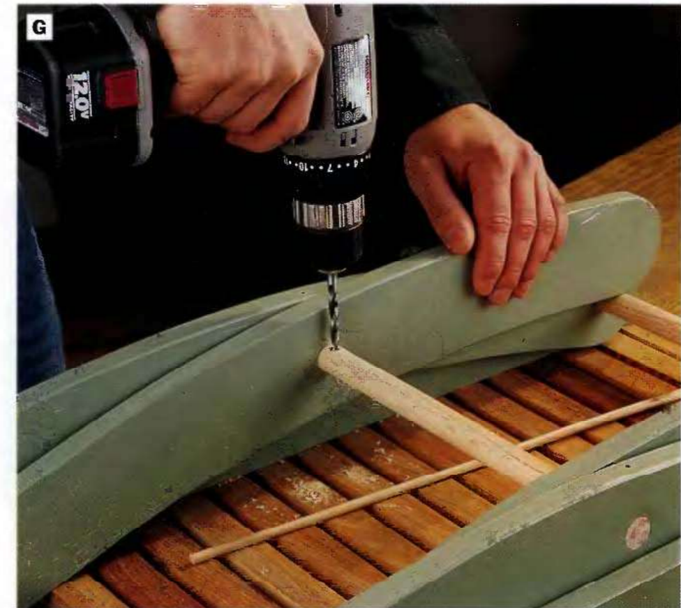
PHOTO G: Lock the inner legs in place by drilling and inserting 1/4-in.-dia. dowels through the leg pivot dowel. Position the lock dowels to leave a slight bit of room between the legs, so they can move easily past one another without damaging the painted finish of the parts.
